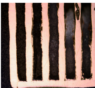
Fig. 10. Vectors with 82.5 Watt power and 0.5 m/s scanning speed
