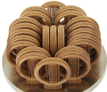
Fig. 43. Set of pavé rings after completion of the production
