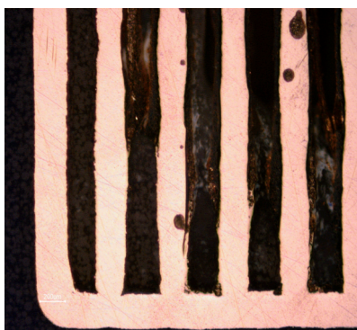
Fig. 13. Vectors with 92.5 Watt power and 80 μs laser exposure time
