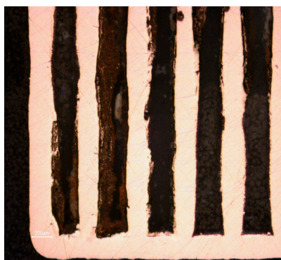
Fig. 9. Vectors with 92.5 Watt power and 0.5 m/s scanning speed
