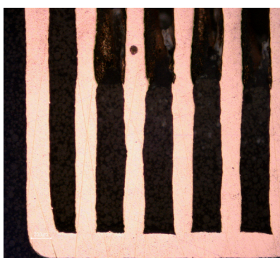
Fig. 14. Vectors with 82.5 Watt power and 80 μs laser exposure time
