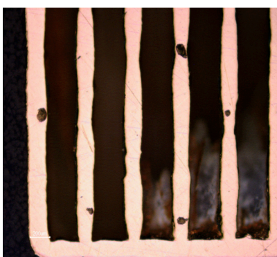
Fig. 11. Vectors with 72.5 Watt power and 0.5 m/s scanning speed
