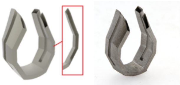
Figure 6 Digital model (left), the section of the model with extended thin areas (center), and photograph of the printed titanium ring (right) with a 0.2 mm wall thickness.
