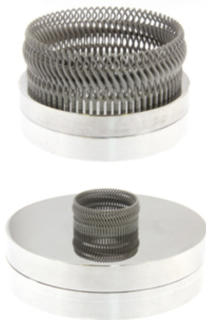
Figure 2 Heart bracelet and ring, 950 platinum, printed by SLM™ (Designer: Xin Xin Zhou, IED Turin—Jewelry and Accessories Design Course)
