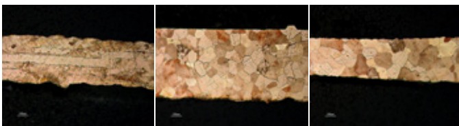
Figure 3 Microstructure of a yellow gold item, obtained by SLM™ (left), traditional investment casting (center) and direct investment casting (right). In the case of SLM™, the measured average grain size is 30 micrometers; with investment casting, it is in the range of 90 micrometers. 5
