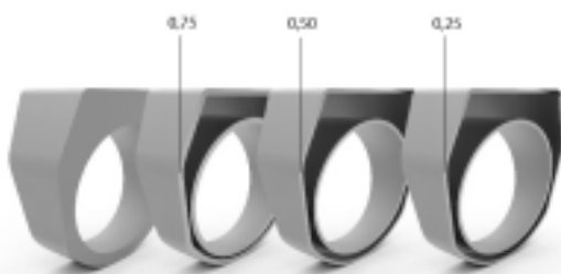
Figure 19 Digital model of the platinum ring at various levels of hollowness
