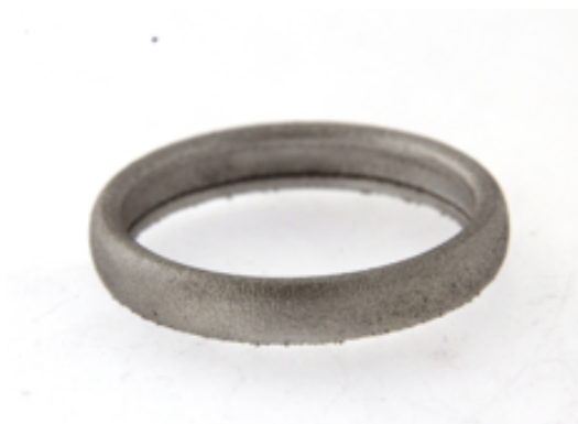
Figure 33 SLM™-produced band model I4 after shot peening
