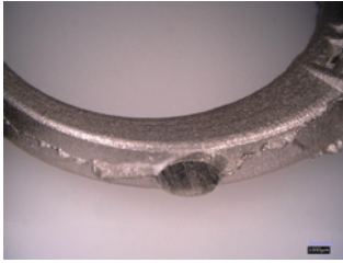
Figure 41 Material excess on the side of the cast ring (fin defect)
