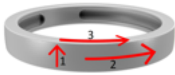
Figure 34 Roughness measurement directions for bands
