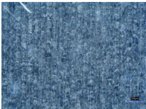
Figure 89 "As-print" SLM™ sample, 200X
