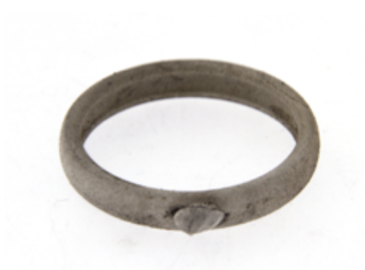
Figure 30 Rough band model 4 produced using casting
