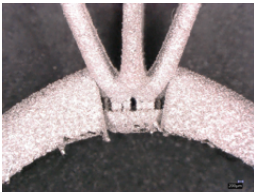
Figure 28 Internal supports of solitaire model 4
