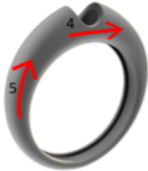
Figure 35 Roughness measurement directions for SLM™ solitaires and trilogies
