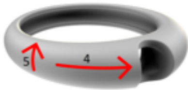
Figure 36 Roughness measurement direction for cast solitaires and trilogies
