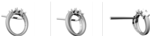
Figure 3 Sequence for removing the interchangeable spring for the Trilogy model
