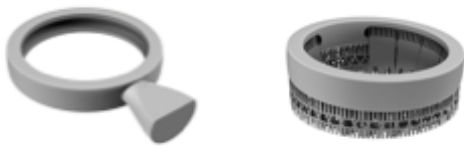
Figure 16 Feeders and supports used for the production of band model 1
