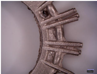
Figure 42 Example of finning caused by investment rupture
