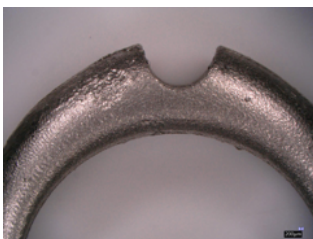
Figure 46 Irregular surface on cast solitaire model 7
