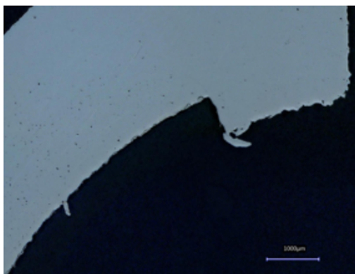
Figure 85 Inter-hatch porosity in a section of an SLM™ ring
