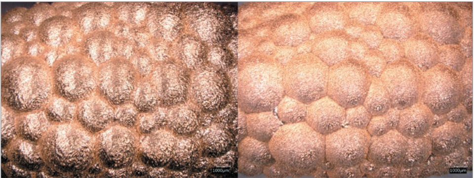
Figure 69 Comparison of bubble details with low- (left) and high-resolution strategy (right)
