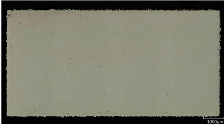
Figure 50 The sample BOX1 of TEST13 shows some internal porosity.
