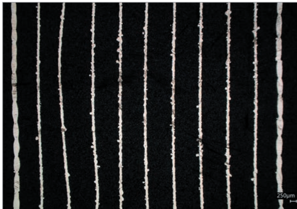
Figure 16 Vector S11 with 44 W and 0.375 m/s from TEST2
