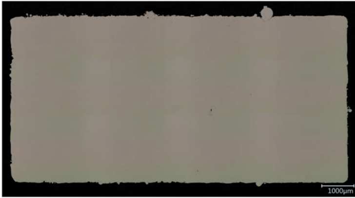
Figure 18 BOX2 (TEST6) after metallographic section
