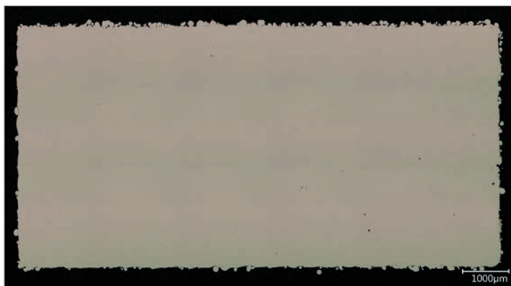
Figure 17 BOX1 (TEST6) after metallographic section
