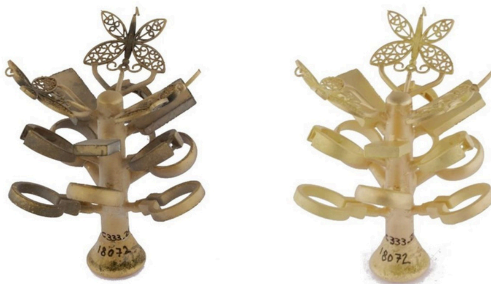
Figure 13: Appearance of reference yellow gold 18K (m-YG) before and after pickling.
