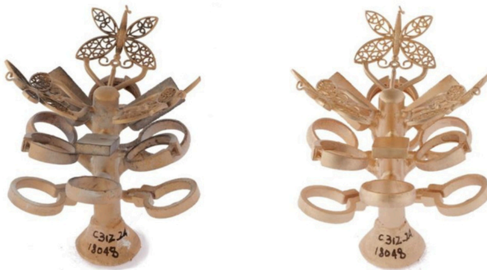
Figure 12: Appearance of reference red gold 18K (m-RG) before and after pickling.
