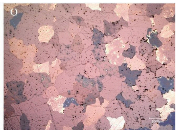
Figure 16. Alloy grains after metallographic etching
