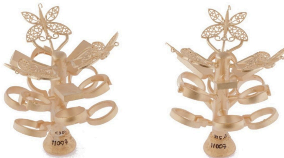
Figure 15: Appearance of red gold 18K with silicon (A) before and after pickling.
