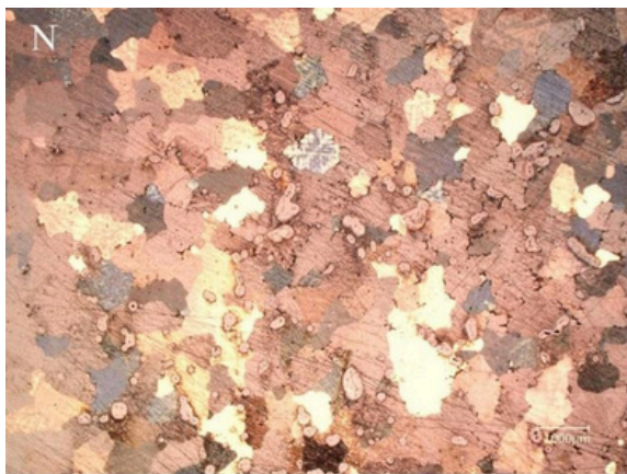
Figure 16. Alloy grains after metallographic etching
