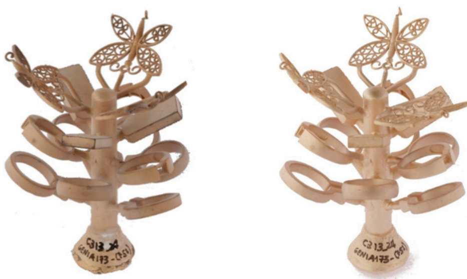
Figure 14: Appearance of refined red gold 18K (r-RG) before and after pickling.
